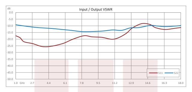
Variable Gain Control Amplifier, 1 GHz to 26.5 GHz, GaAs FET, 40 dB Gain, 20 dB Variable Gain, +13 dBm P1dB, SMA from Fairview Microwave is in-stock and available to ship same-day. All of our RF/microwave products are available off-the-shelf from our ISO 9001:2008 certified facilities in Lewisville, Texas. Fairview Microwave is RF on-demand.
