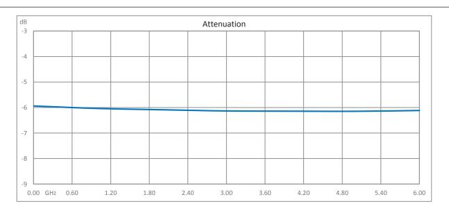
6 dB Fixed Attenuator SMA Male (Plug) To SMA Female (Jack) From 0.009 MHz To 6 GHz Rated To 2 Watts, Copper Body, 1.15 VSWR from Fairview Microwave is in-stock and available to ship same-day. All of our RF/microwave products are available off-the-shelf from our ISO 9001:2008 certified facilities in Lewisville, Texas. Fairview Microwave is RF on-demand.
