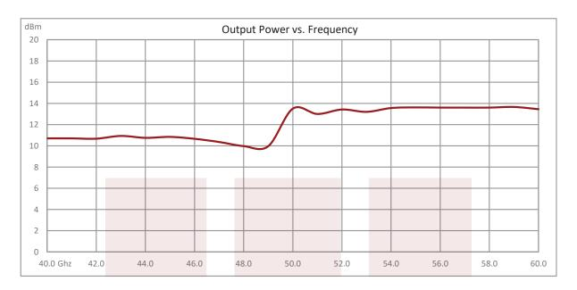
40 GHz to 60 GHz U-Band 4x Active Frequency Multiplier, +10 dBm Pout, WR-19 Output with UG-383/U-M Flange, SMA Female Input from Fairview Microwave is in-stock and available to ship same-day. All of our RF/microwave products are available off-the-shelf from our ISO 9001:2008 certified facilities in Lewisville, Texas. Fairview Microwave is RF on-demand.
