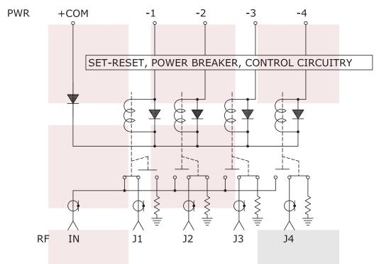
SCHEMATIC LATCHING WITH 50 OHM TERMINATION SHOWN IN POSITION 1 (COM - J1)
