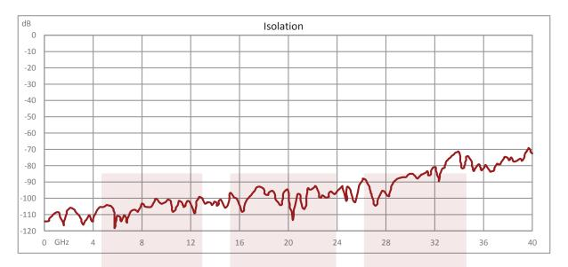
SP4T Latching 0.05 dB Low Insertion Loss Repeatability DC to 40 GHz Terminated Relay Switch, Indicators, Self Cut Off, 5W, 24V, 2.92mm from Fairview Microwave is in-stock and available to ship same-day. All of our RF/microwave products are available off-the-shelf from our ISO 9001:2008 certified facilities in Allen, Texas. Fairview Microwave is RF on-demand.
