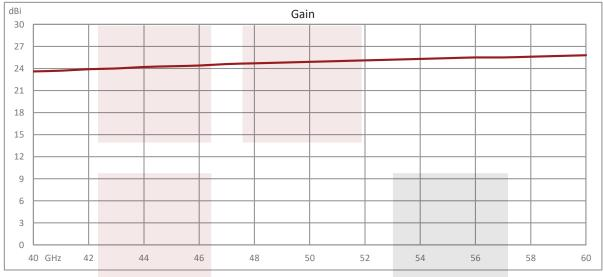
Standard Gain Horn Waveguide Antenna, WR-19, 40 GHz to 60 GHz, UG-383/U-Mod Round Cover Flange, 25 dBi Nominal Gain from Fairview Microwave is in-stock and available to ship same-day. All of our RF/microwave products are available off-the-shelf from our ISO 9001:2008 certified facilities in Allen, Texas. Fairview Microwave is RF on-demand.
