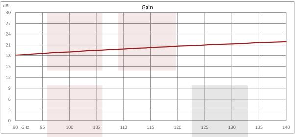
Standard Gain Horn Waveguide Antenna, WR-8, 90 GHz to 140 GHz, UG-387/U-Mod Round Cover Flange, 20 dBi Nominal Gain from Fairview Microwave is in-stock and available to ship same-day. All of our RF/microwave products are available off-the-shelf from our ISO 9001:2008 certified facilities in Allen, Texas. Fairview Microwave is RF on-demand.
