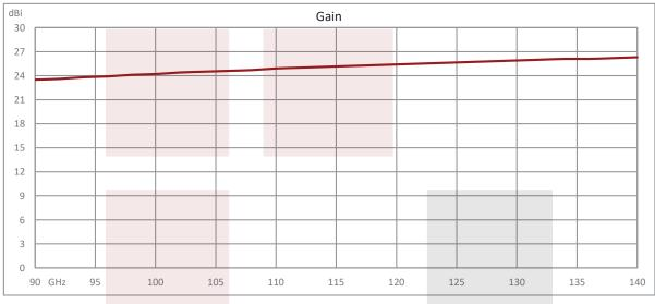
Standard Gain Horn Waveguide Antenna, WR-8, 90 GHz to 140 GHz, UG-387/U-Mod Round Cover Flange, 25 dBi Nominal Gain from Fairview Microwave is in-stock and available to ship same-day. All of our RF/microwave products are available off-the-shelf from our ISO 9001:2008 certified facilities in Allen, Texas. Fairview Microwave is RF on-demand.
