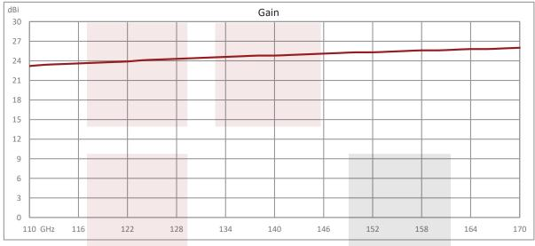
Standard Gain Horn Waveguide Antenna, WR-6, 110 GHz to 170 GHz, UG-387/U-Mod Round Cover Flange, 25 dBi Nominal Gain from Fairview Microwave is in-stock and available to ship same-day. All of our RF/microwave products are available off-the-shelf from our ISO 9001:2008 certified facilities in Allen, Texas. Fairview Microwave is RF on-demand.
