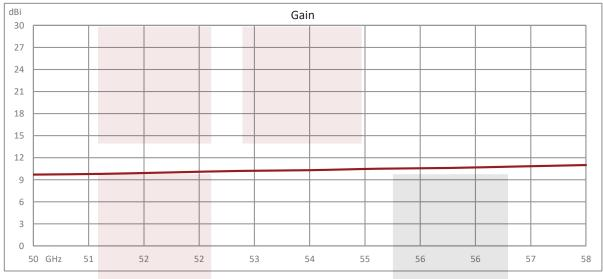
Conical Gain Horn Waveguide Antenna, WR-19, 50 GHz to 58 GHz, UG-383/U-Mod Round Cover Flange, 10 dBi Nominal Gain from Fairview Microwave is in-stock and available to ship same-day. All of our RF/microwave products are available off-the-shelf from our ISO 9001:2008 certified facilities in Allen, Texas. Fairview Microwave is RF on-demand.
