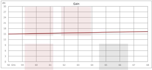
Conical Gain Horn Waveguide Antenna, WR-15, 58 GHz to 68 GHz, UG-385/U Round Cover Flange, 15 dB Nominal Gain from Fairview Microwave is in-stock and available to ship same-day. All of our RF/microwave products are available off-the-shelf from our ISO 9001:2008 certified facilities in Allen, Texas. Fairview Microwave is RF on-demand.
