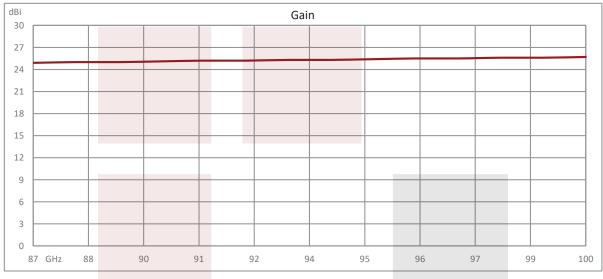
Conical Gain Horn Waveguide Antenna, WR-10, 87 GHz to 100 GHz, UG-387/U Round Cover Flange, 25 dBi Nominal Gain from Fairview Microwave is in-stock and available to ship same-day. All of our RF/microwave products are available off-the-shelf from our ISO 9001:2008 certified facilities in Allen, Texas. Fairview Microwave is RF on-demand.
