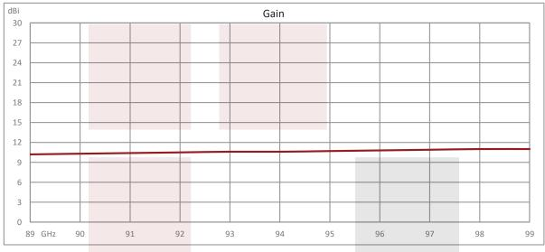
Wide Angle Scalar Feed Horn Waveguide Antenna, WR-10, 89 GHz to 99 GHz, UG-385/U-Mod Round Cover Flange, 10 dBi Nominal Gain from Fairview Microwave is in-stock and available to ship same-day. All of our RF/microwave products are available off-the-shelf from our ISO 9001:2008 certified facilities in Allen, Texas. Fairview Microwave is RF on-demand.
