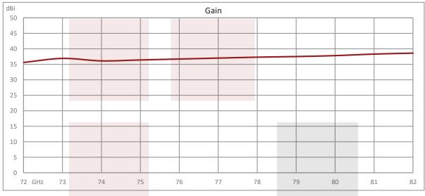
Lens Horn Waveguide Antenna, WR-12, 72 GHz to 82 GHz, UG-387/U Round Cover Flange, 37 dBi Nominal Gain from Fairview Microwave is in-stock and available to ship same-day. All of our RF/microwave products are available off-the-shelf from our ISO 9001:2008 certified facilities in Allen, Texas. Fairview Microwave is RF on-demand.
