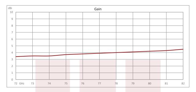
Omni-directional Waveguide Antenna, WR-12, 75 GHz to 79 GHz, UG-387/U Round Cover Flange, 2 dBi Nominal Gain from Fairview Microwave is in-stock and available to ship same-day. All of our RF/microwave products are available off-the-shelf from our ISO 9001:2008 certified facilities in Allen, Texas. Fairview Microwave is RF on-demand.
