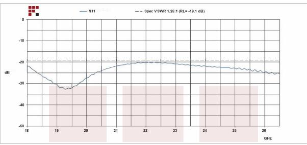
WR-42 to 2.92mm Female Waveguide to Coax Adapter UG-597/U Square Cover with 18 GHz to 26.5 GHz K Band in Aluminum, Chem Film from Fairview Microwave is in-stock and available to ship same-day. All of our RF/microwave products are available off-the-shelf from our ISO 9001:2008 certified facilities in Allen, Texas. Fairview Microwave is RF on-demand.
