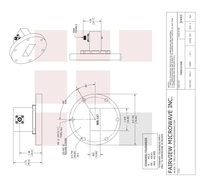
WR-137 to SMA Female Waveguide to Coax Adapter UG-441/U Round Cover with  $5.85~\mathrm{GHz}$  to  $8.2~\mathrm{GHz}$  C Band in Aluminum, Paint
