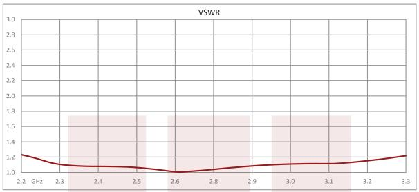
WR-340 to Type N Female Waveguide to Coax Adapter CPR-340G Grooved with 2.2 GHz to 3.3 GHz F Band in Aluminum, Paint from Fairview Microwave is in-stock and available to ship same-day. All of our RF/microwave products are available off-the-shelf from our ISO 9001:2008 certified facilities in Allen, Texas. Fairview Microwave is RF on-demand.
