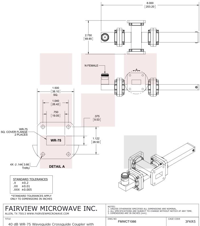
40 dB WR-75 Waveguide Crossguide Coupler with Square Cover Flange and N Female Coupled Port from 10 GHz to 15 GHz in Bronze
