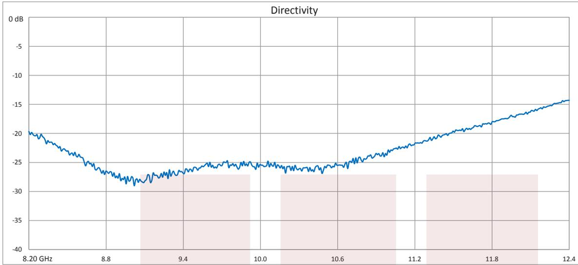
20 dB WR-90 Waveguide Crossguide Coupler with CPR-90G Flange and SMA Female Coupled Port from 8.2 GHz to 12.4 GHz in Bronze from Fairview Microwave is in-stock and available to ship same-day. All of our RF/microwave products are available off-the-shelf from our ISO 9001:2008 certified facilities in Allen, Texas. Fairview Microwave is RF on-demand.
