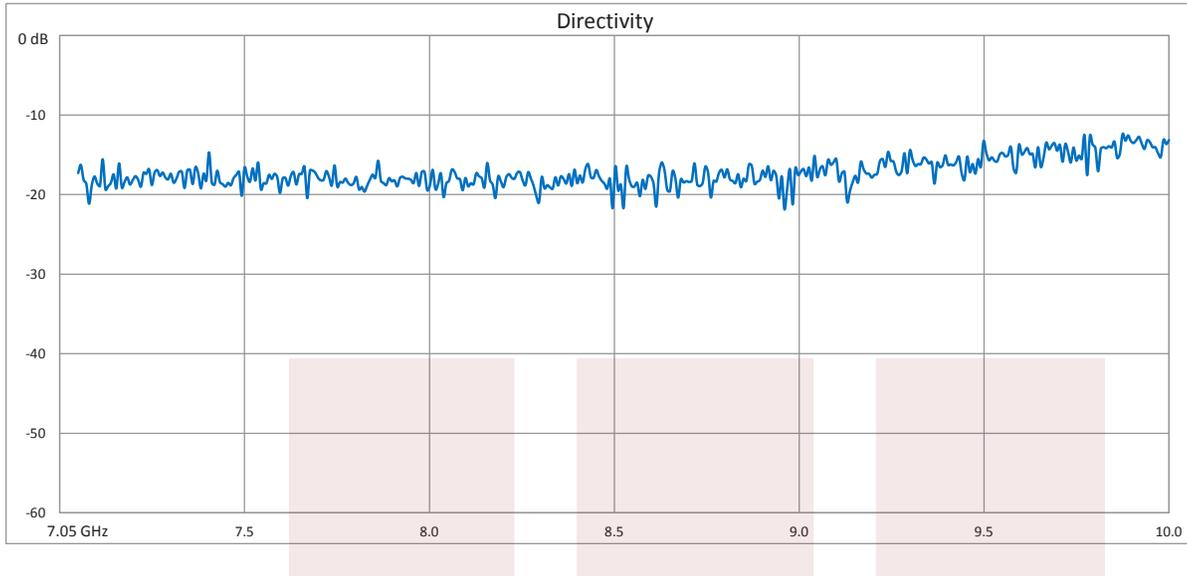
40 dB WR-112 Waveguide Crossguide Coupler with CPR-112G Flange and N Female Coupled Port from 7.05 GHz to 10 GHz in Bronze from Fairview Microwave is in-stock and available to ship same-day. All of our RF/microwave products are available off-the-shelf from our ISO 9001:2008 certified facilities in Allen, Texas. Fairview Microwave is RF on-demand.
