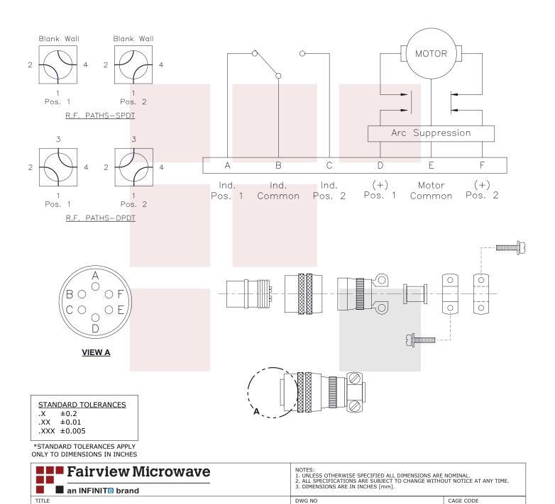
WRD-180 Double Ridge Waveguide Latching Relay Switch SPDT/DPDT, 18 GHz to 40 GHz Frequency Band, 2,000 Watts, UG Cover, 12V, Self Cut Off
