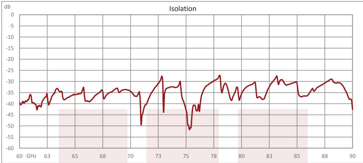
WR-12 Waveguide Isolator with 25 dB min Isolation from 60 GHz to 90 GHz using Round Cover UG-387/U Flange from Fairview Microwave is in-stock and available to ship same-day. All of our RF/microwave products are available off-the-shelf from our ISO 9001:2008 certified facilities in Allen, Texas. Fairview Microwave is RF on-demand.
