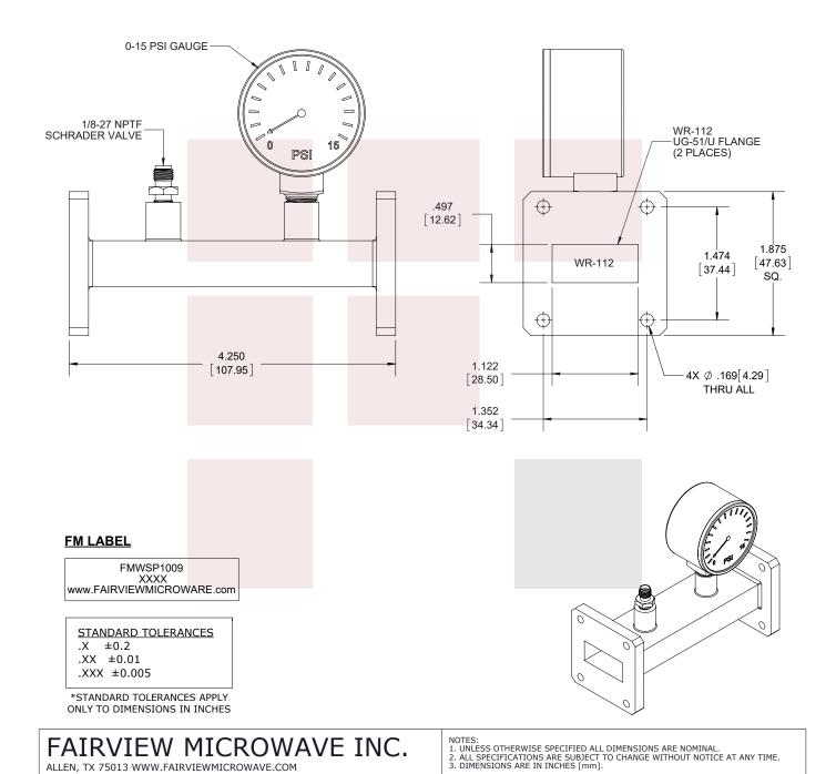
WR-112 Waveguide Pressurizing Section 4.25 Inch Length With UG-51/U Square Cover Flange from 7.05
