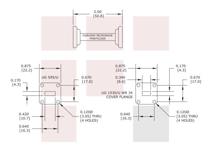
$\begin{array}{cc} \underline{\text{STANDARD TOLERANCES}} \\ .\text{X} & \pm 0.2 \\ .\text{XX} & \pm 0.1 \end{array}$
