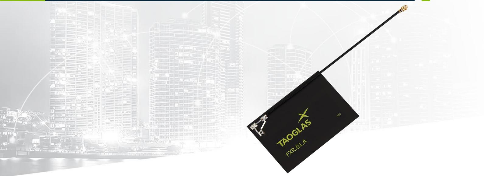
Taoglas has developed an NFC (Near Field Communications) antenna for use with NFC readers. This standard design is matched to a 50 Ohm system and provides a well-matched solution for NFC readers. The antenna is dimensioned to provide the capability of interrogating typical size NFC tags out to a 5 cm. distance. This standard antenna is delivered with a coaxial cable connected to the antenna element to ease use and integration into customer devices.
