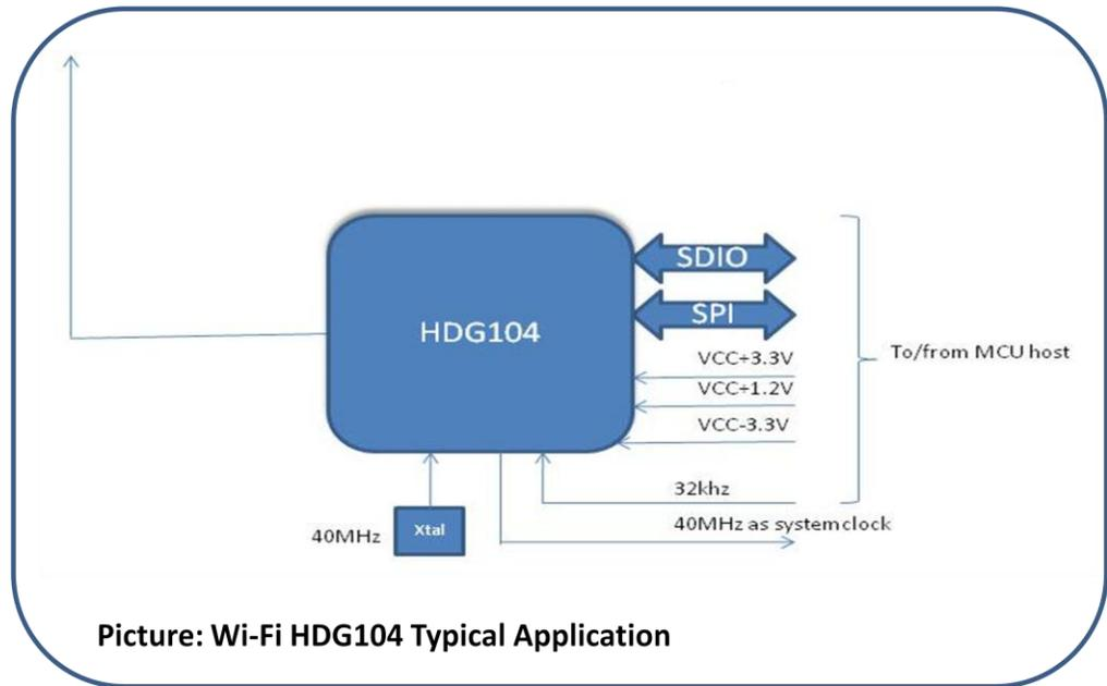
Picture: Wi-Fi HDG104 Typical Application
