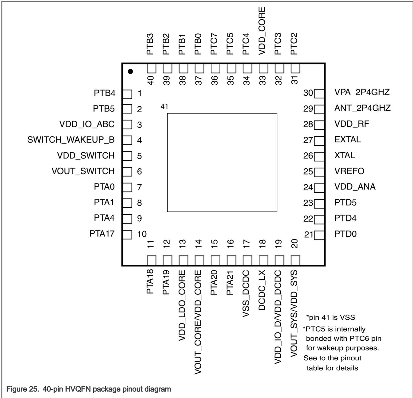
Figure 25. 40-pin HVQFN package pinout diagram
