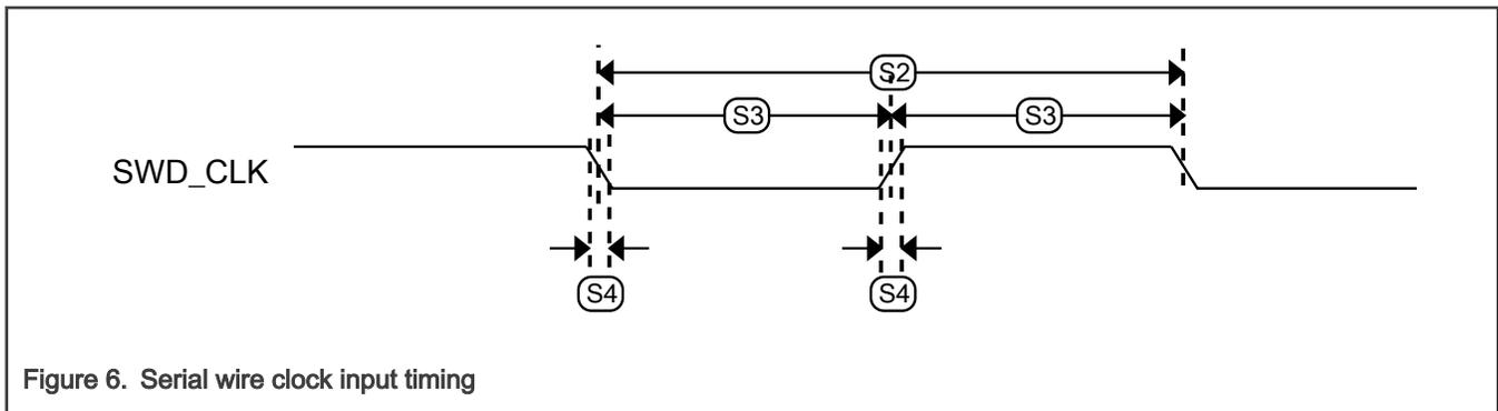
Figure 6. Serial wire clock input timing
