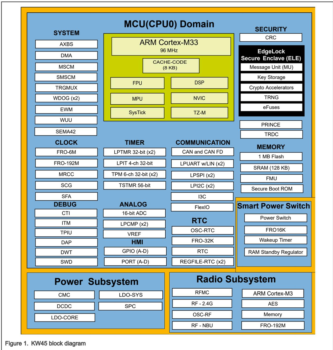
Figure 1. KW45 block diagram
