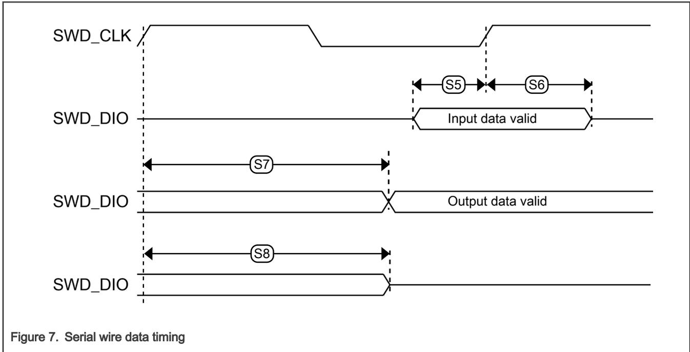
Figure 7. Serial wire data timing
