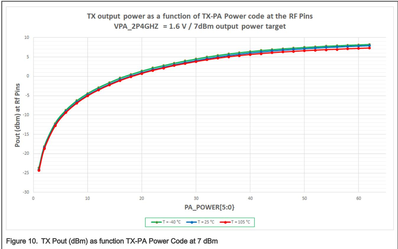
Figure 10. TX Pout (dBm) as function TX-PA Power Code at 7 dBm
