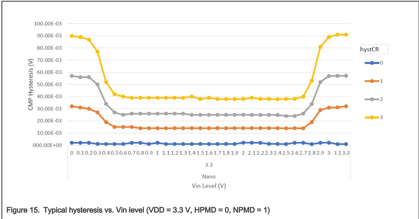
Figure 15. Typical hysteresis vs. Vin level (VDD = 3.3 V, HPMD = 0, NPMD = 1)
