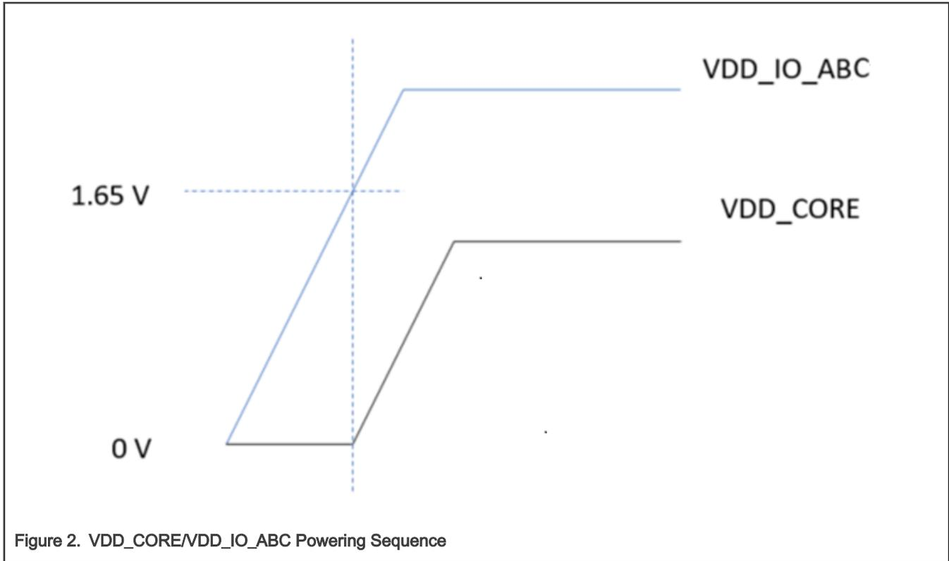
Figure 2. VDD\_CORE/VDD\_IO\_ABC Powering Sequence
