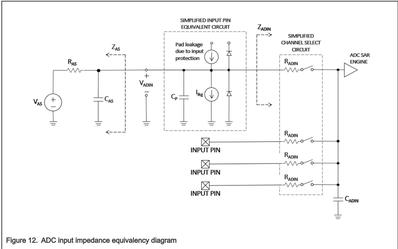
Figure 12. ADC input impedance equivalency diagram
