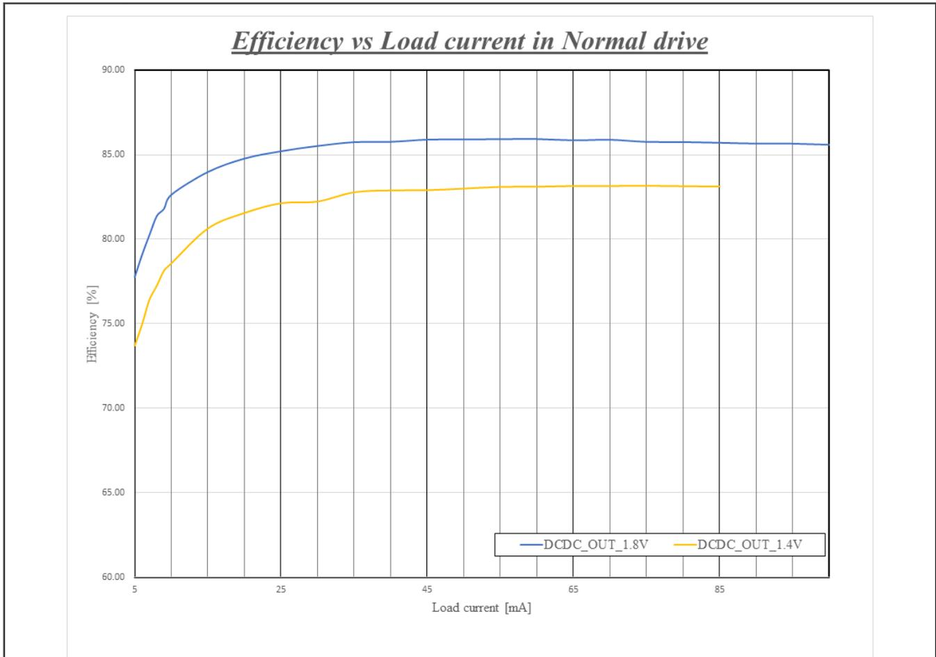
Figure 4. Efficiency vs Load current in Normal drive
