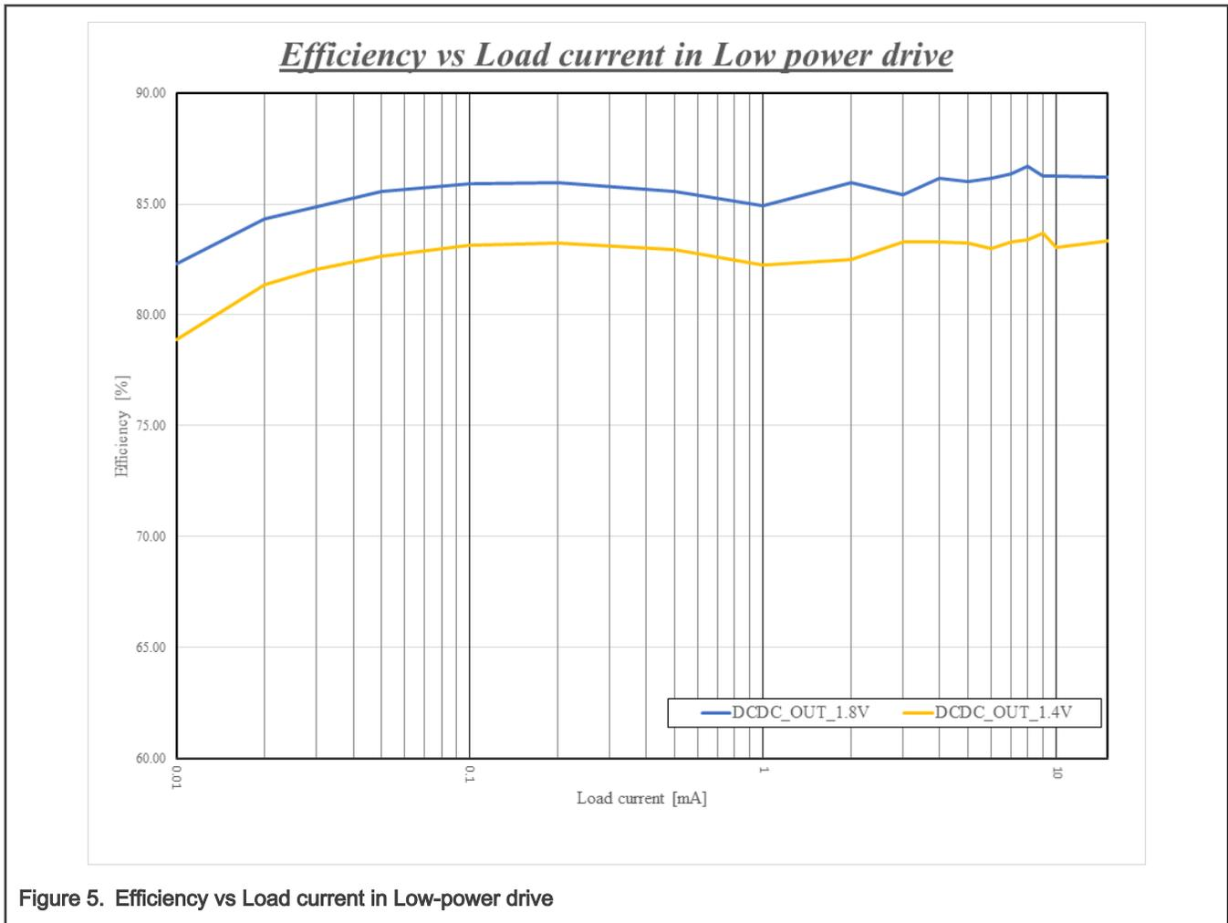
Figure 5. Efficiency vs Load current in Low-power drive
