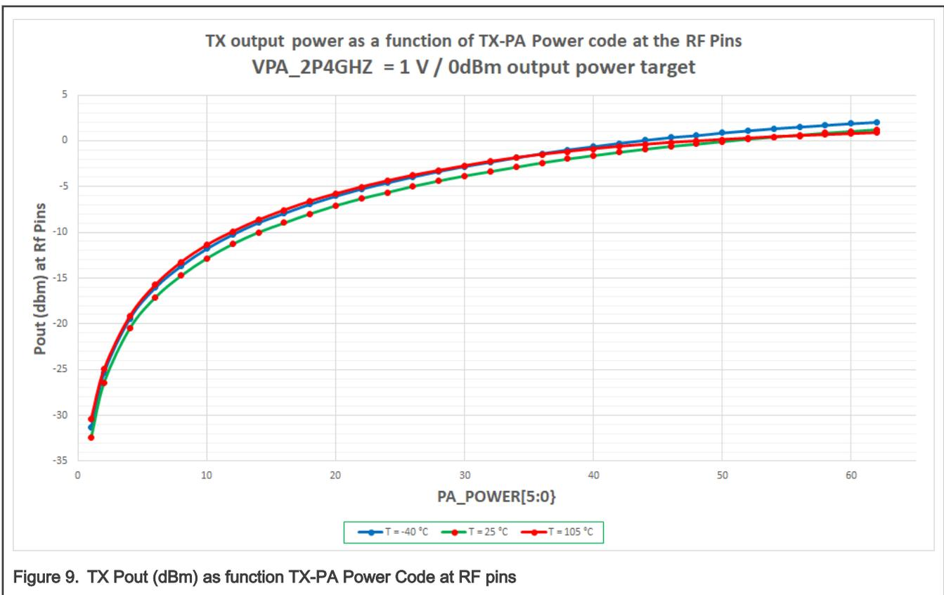
Figure 9. TX Pout (dBm) as function TX-PA Power Code at RF pins
