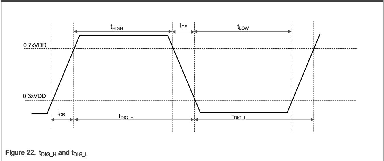
Figure 22.  $t_{DIG\_H}$  and  $t_{DIG\_L}$
