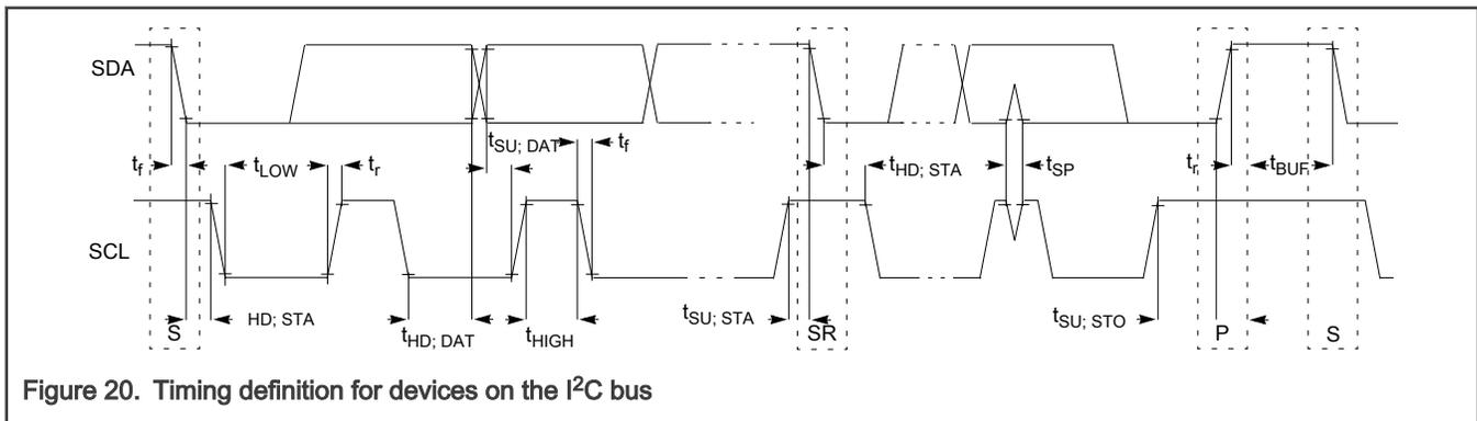
**Figure 20. Timing definition for devices on the I<sup>2</sup>C bus**
