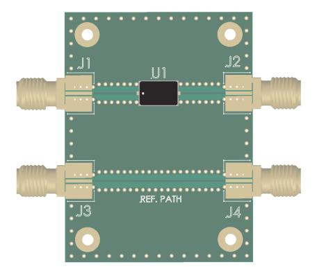
The evaluation board for the LM202402-Q-x-301 limiter is shown above. This evaluation board comprises two sections: the evaluation circuit for the limiter module; and, a reference transmission line.
