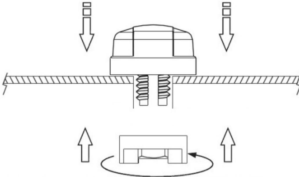
Recommended torque for Mounting is 24.5N·m
