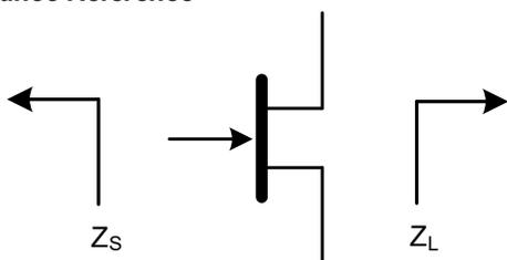
Z<sub>SOURCE</sub> = Measured impedance presented to the input of the device at package reference plane.
