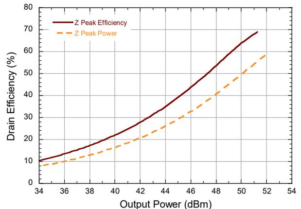
28 V Pulsed<sup>4</sup> Load-Pull Performance (Per Each Side of Symmetric Device)
