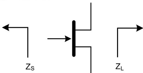
Z<sub>SOURCE</sub> = Measured impedance presented to the input of the device at package reference plane.
