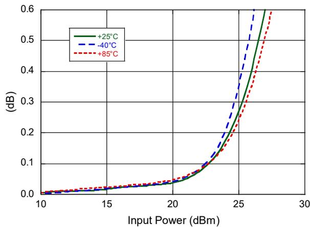
**Compression Power, over Temperature @ 18 GHz,  $V_R = -2$  V**
