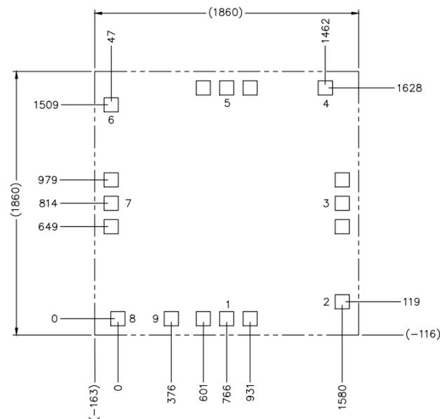
6. Bond pad dimensions 1 - 7, 100 μm x 100 μm .
