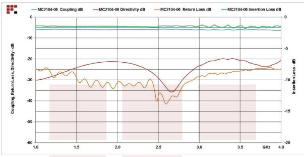
SMA Directional Coupler 6 dB Coupled Port From 1 GHz to 4 GHz Rated To 50 Watts from Fairview Microwave is in-stock and available to ship same-day. All of our RF/microwave products are available off-the-shelf from our ISO 9001:2008 certified facilities in Lewisville, Texas. Fairview Microwave is RF on-demand.
