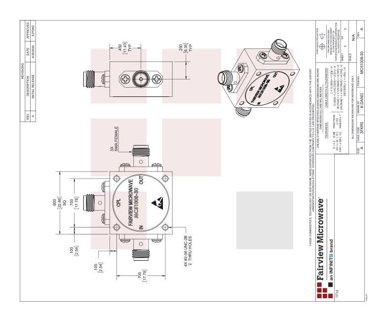
SMA Directional Coupler 30 dB Coupled Port From 5 MHz to 1,000 MHz Rated To 3 Watts
