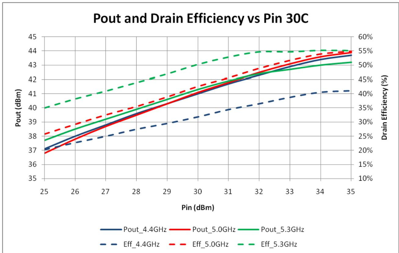
**Typical RF Performance(Cont'l):**  $V_{ds}=28.0V, V_{gs}=-2.84, I_{dq}=140mA, Z_0=50\text{ ohm}, T_a=25\text{ }^\circ\text{C}$
