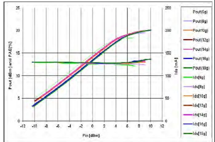
Pout[dBm], Gain[dB], and Ids[mA] vs. Input power [dBm]
