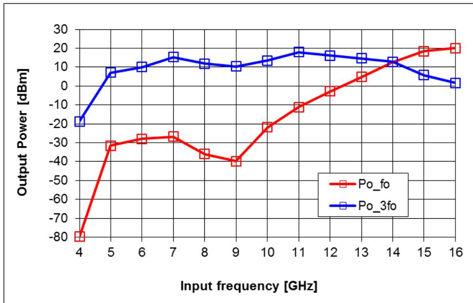
Measured 3x multiplier data: Pin=9dBm, Vd1=1V, Vd2=5V, Vg1=-0.75V, Vg2=-0.75V, Id1=21mA, and Id2=144mA
