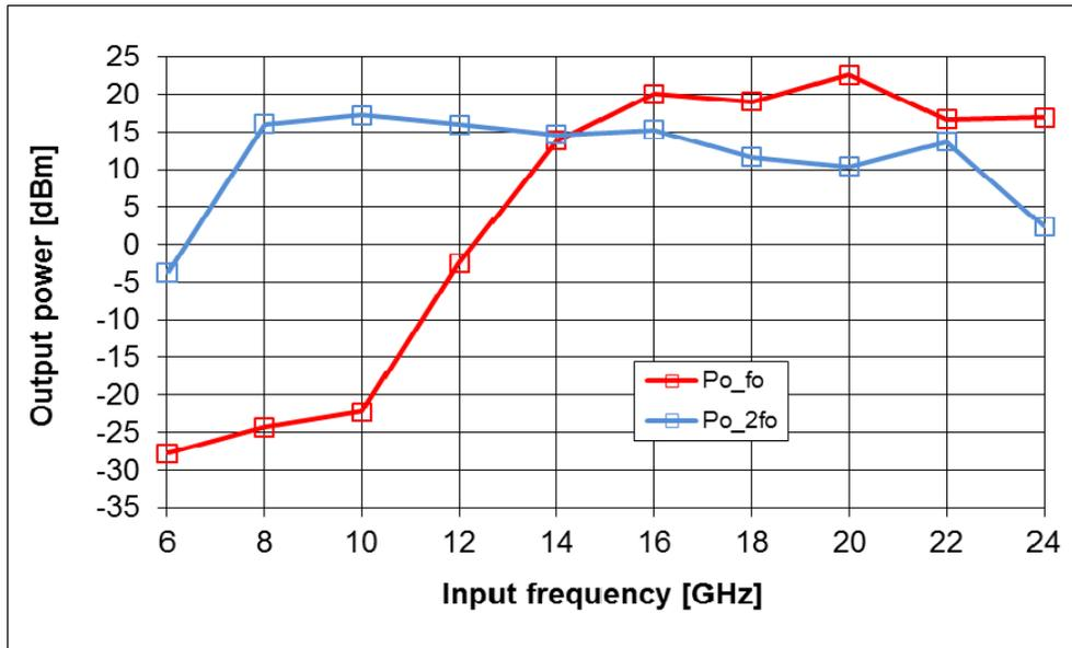
Measured 2x multiplier data: Pin=9dBm, Vd1=5V, Vd2=5V, Vg1=-1.4V, Vg2=-0.7V, Id1=1mA, and Id2=163mA
