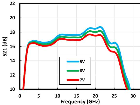
Figure 1-32. Gain vs.  $V_{DD}$  at 120 mA
