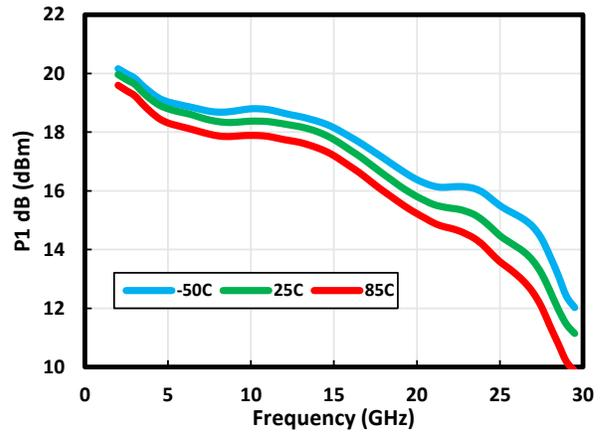
Figure 1-19. P<sub>sat</sub> vs. Temperature at 5V/100 mA
