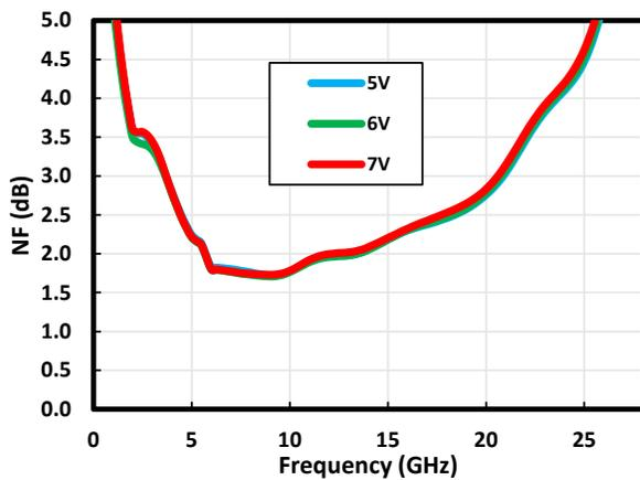
Figure 1-36. NF vs.  $V_{DD}$  at 130 mA
