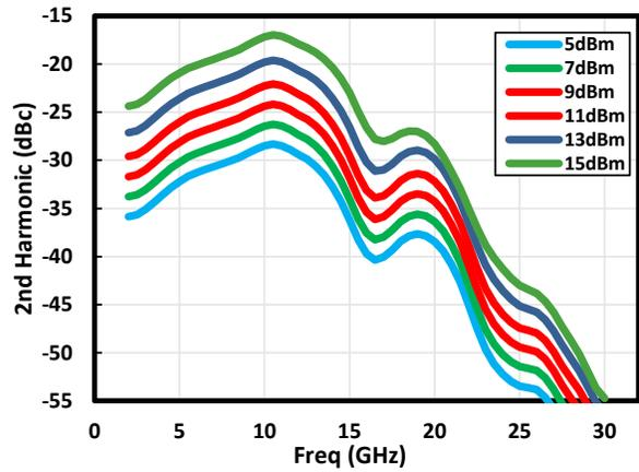
Figure 1-52. 2-nd Harmonic vs. Power at 7V/130 mA
