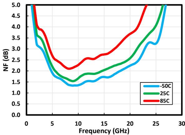
Figure 1-14. NF vs. Temperature at 6V/120 mA
