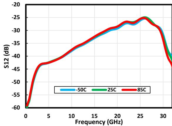
Figure 1-11. S12 vs. Temperature at 6V/120 mA
