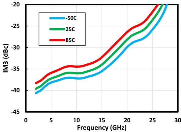
Figure 1-30. IM3 vs. Temperature at 7V/140 mA,
