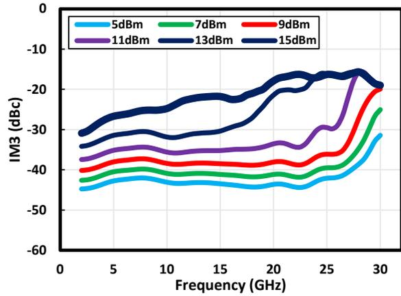
Figure 1-48. IM3 vs. Power at 6V/120 mA
