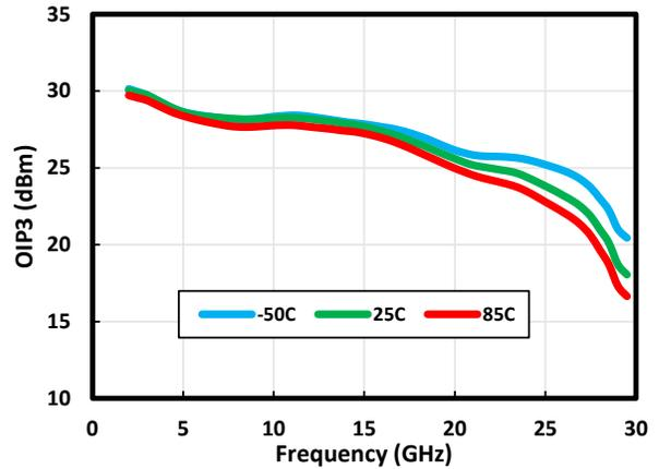
Figure 1-23. OIP3 vs. Temperature at 6V/120 mA
