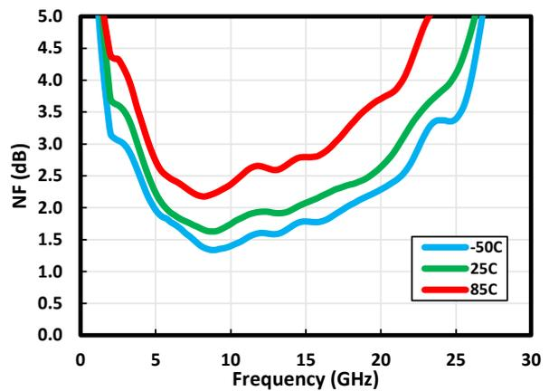
Figure 1-15. NF vs. Temperature at 7V/130 mA
