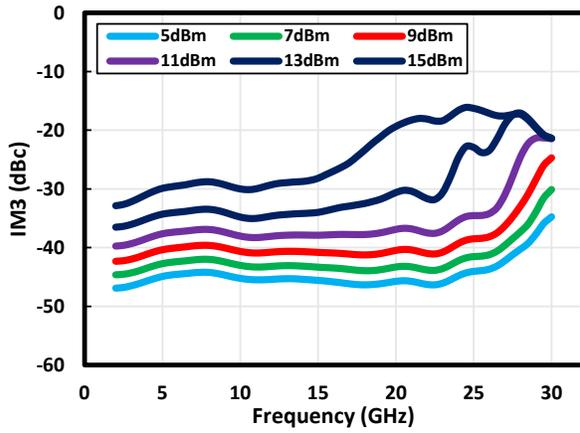
Figure 1-49. IM3 vs. Power at 7V/130 mA
