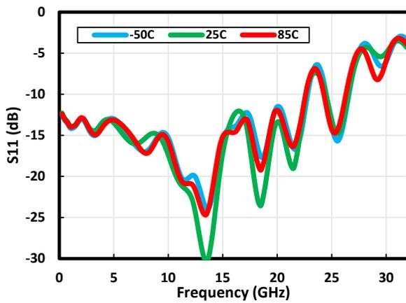
Figure 1-6. S11 vs. Temperature at 7V/130 mA
