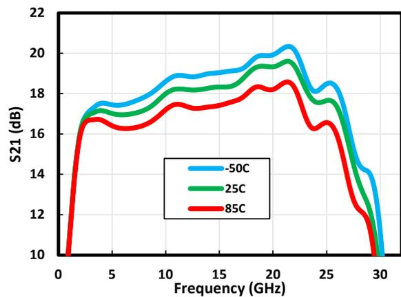
Figure 1-3. Gain vs. Temperature at 7V/130 mA
