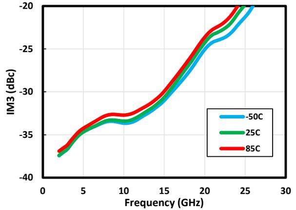
Figure 1-29. IM3 vs. Temperature at 6V/120 mA,
