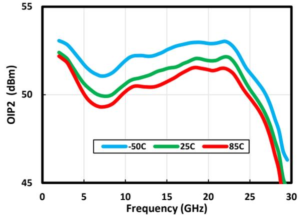
Figure 1-27. OIP2(low) vs. Temperature at 7V/140 mA
