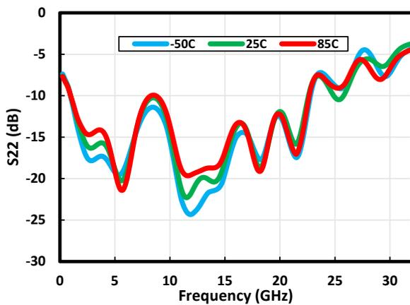
Figure 1-8. S22 vs. Temperature at 6V/120 mA
