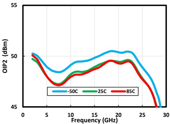
Figure 1-26. OIP2(low) vs. Temperature at 6V/120 mA
