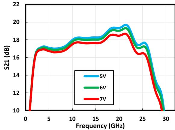
Figure 1-33. Gain vs.  $V_{DD}$  at 130 mA
