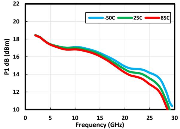
Figure 1-17. P1dB vs. Temperature at 6V/120 mA
