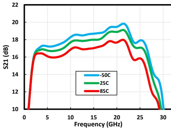
**Figure 1-2.** Gain vs. Temperature at 6V/120 mA
