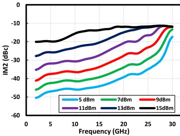
**Figure 1-45. IM2 vs. Power at 6V/120 mA**
