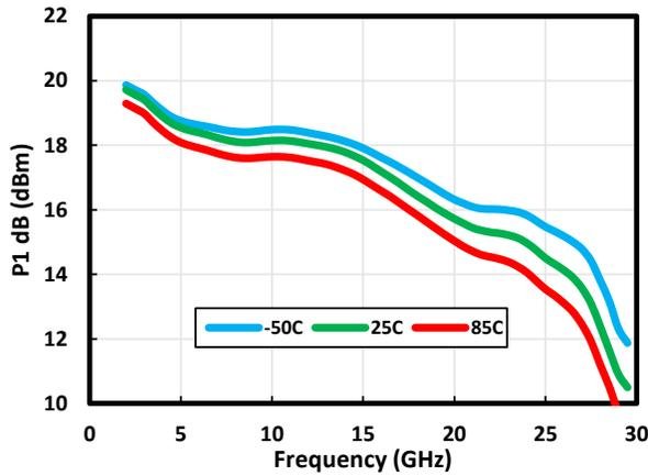
Figure 1-18. P1dB vs. Temperature at 7V/130 mA
