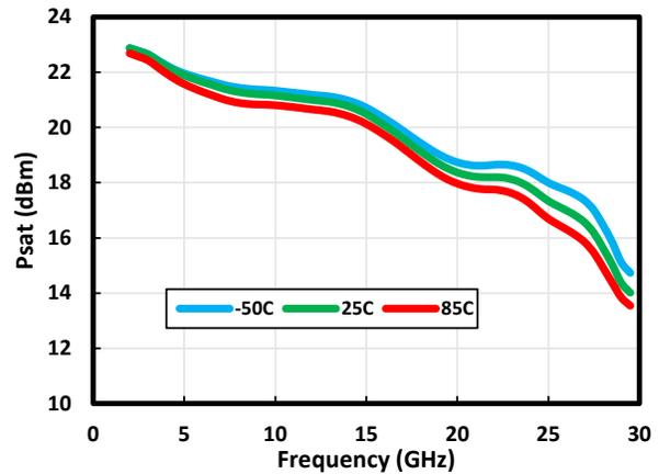
Figure 1-21.  $P_{sat}$  vs. Temperature at 7V/130 mA
