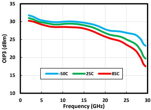
Figure 1-24. OIP3 vs. Temperature at 7V/130 mA
