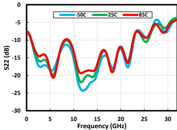
Figure 1-9. S22 vs. Temperature at 7V/130 mA
