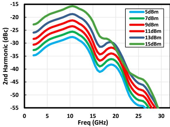
Figure 1-51. 2-nd Harmonic vs. Power at 6V/120 mA
