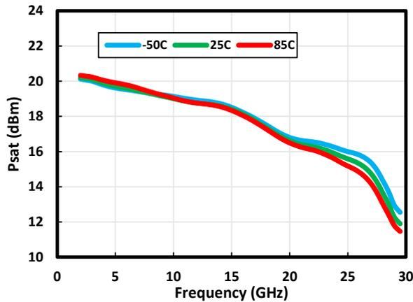
Figure 1-20. P<sub>sat</sub> vs. Temperature at 6V/120 mA
