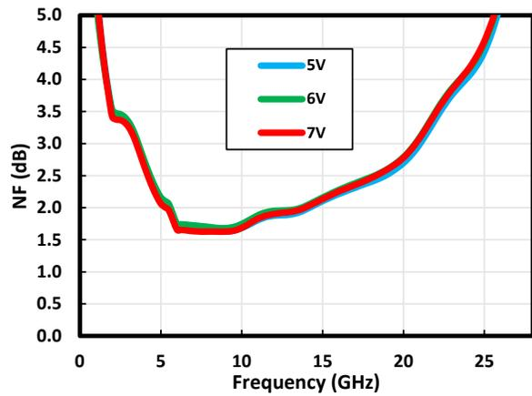
Figure 1-35. NF vs.  $V_{DD}$  at 120 mA
