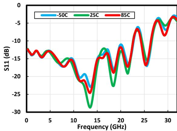
Figure 1-5. S11 vs. Temperature at 6V/120 mA
