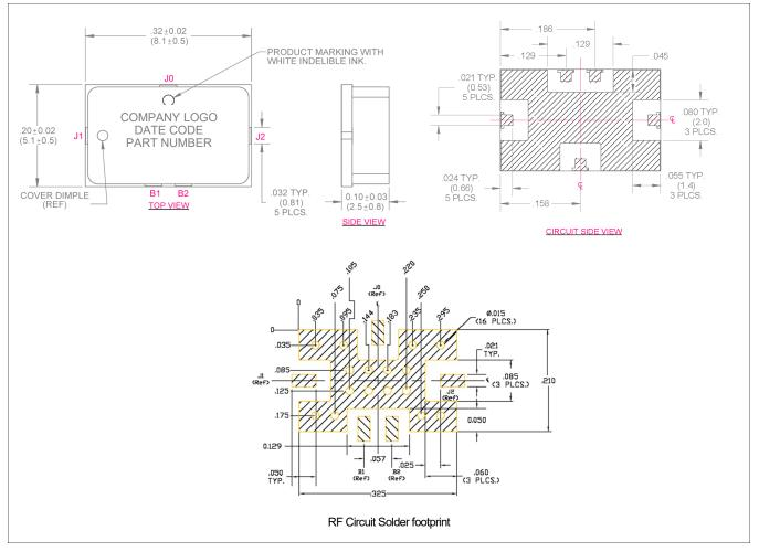
10. Hatched metal area on circuit side of device is RF, DC and thermal grounded.
