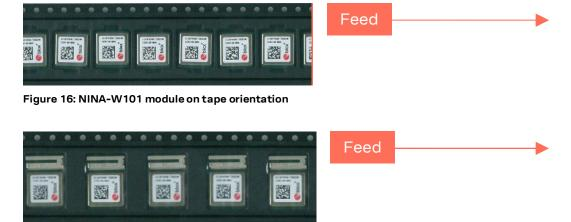
Figure 17: NINA-W102/NINA-W106 module on tape orientation
