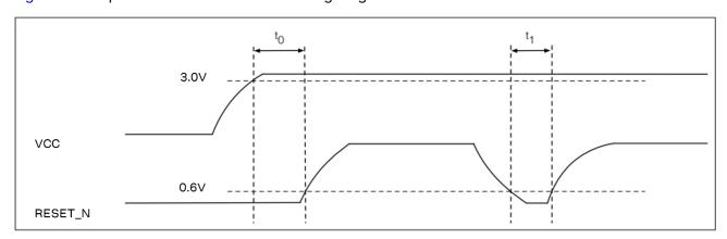
Figure 4: Module power-up and reset timing
