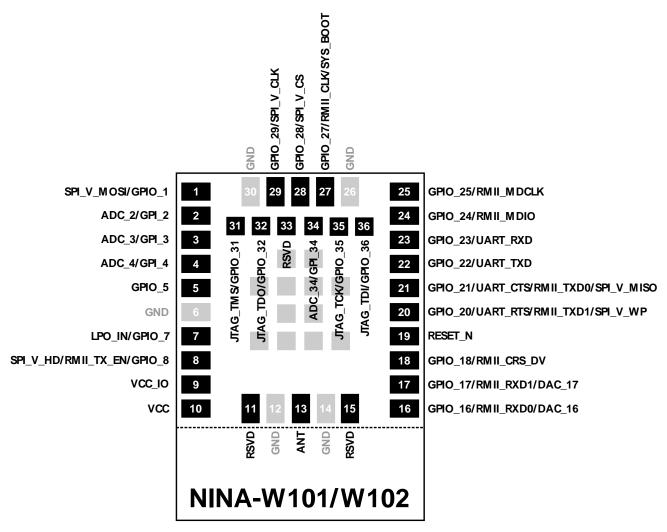
Figure 2: NINA-W101/W102 pin assignment (top view)
