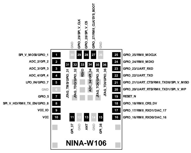
Figure 3: NINA-W106 pin assignment (top view)
