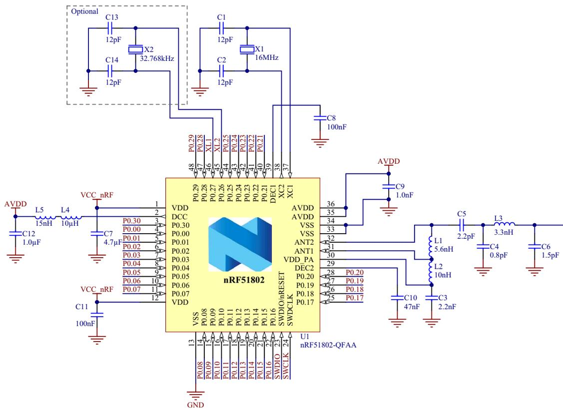
**Figure 21** QFAA QFN48 with DC/DC converter setup
