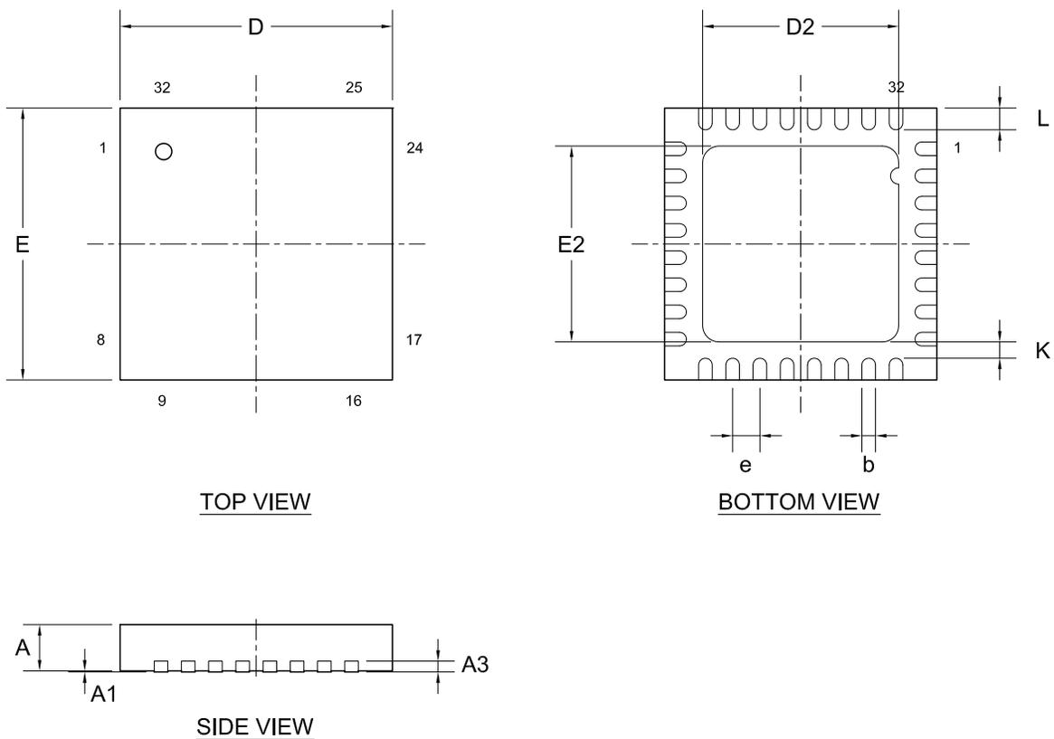
**Figure 15** QFN32 5 x 5 mm package
