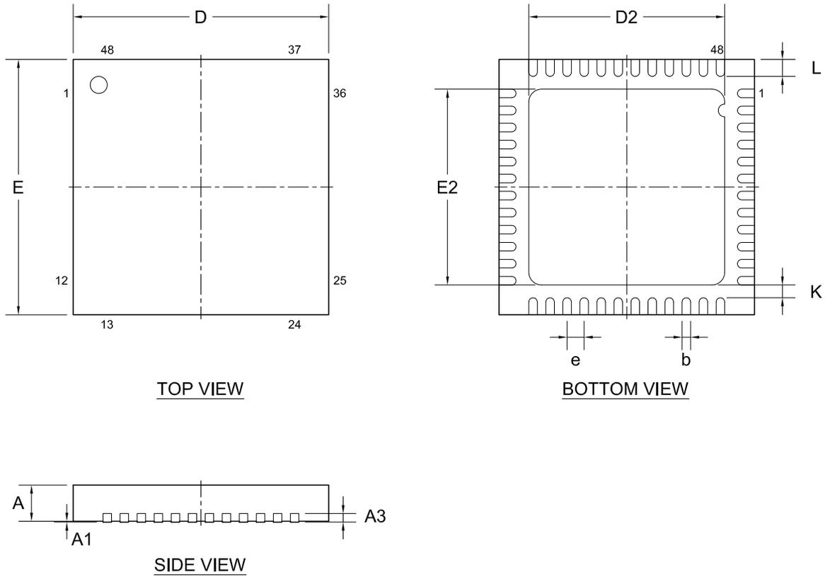
**Figure 14** QFN48 6 x 6 mm package
