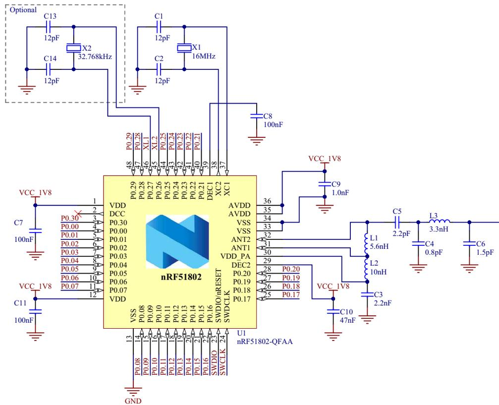
**Figure 20** QFAA QFN48 with low voltage mode setup
