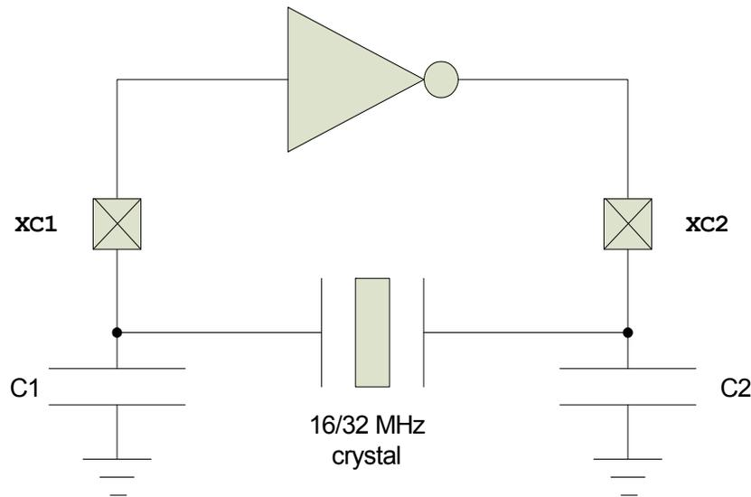
**Figure 6** Circuit diagram of the 16/32 MHz crystal oscillator
