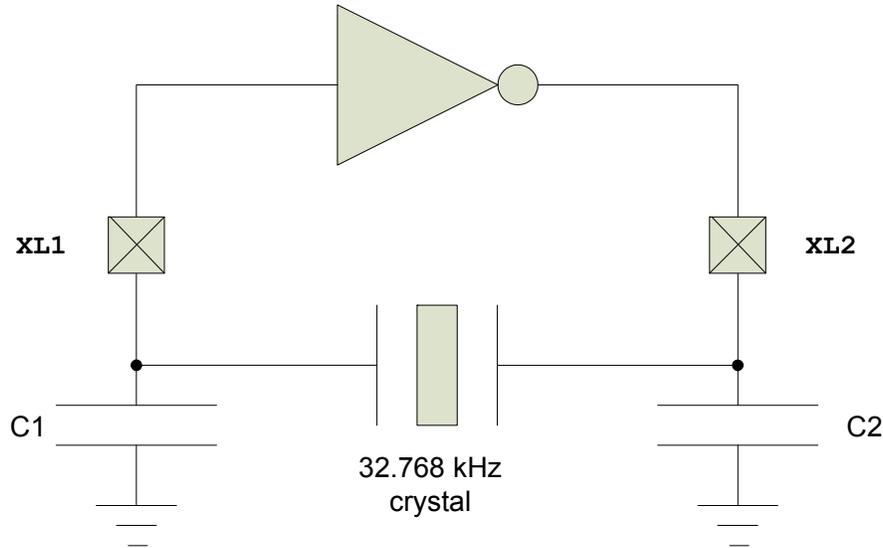
**Figure 7** Circuit diagram of the 32.768 kHz crystal oscillator
