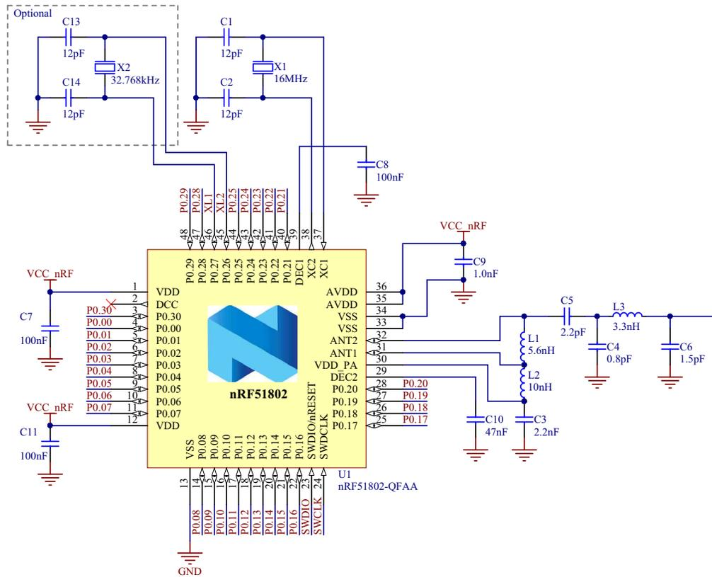
**Figure 19** QFAA QFN48 with internal LDO setup
