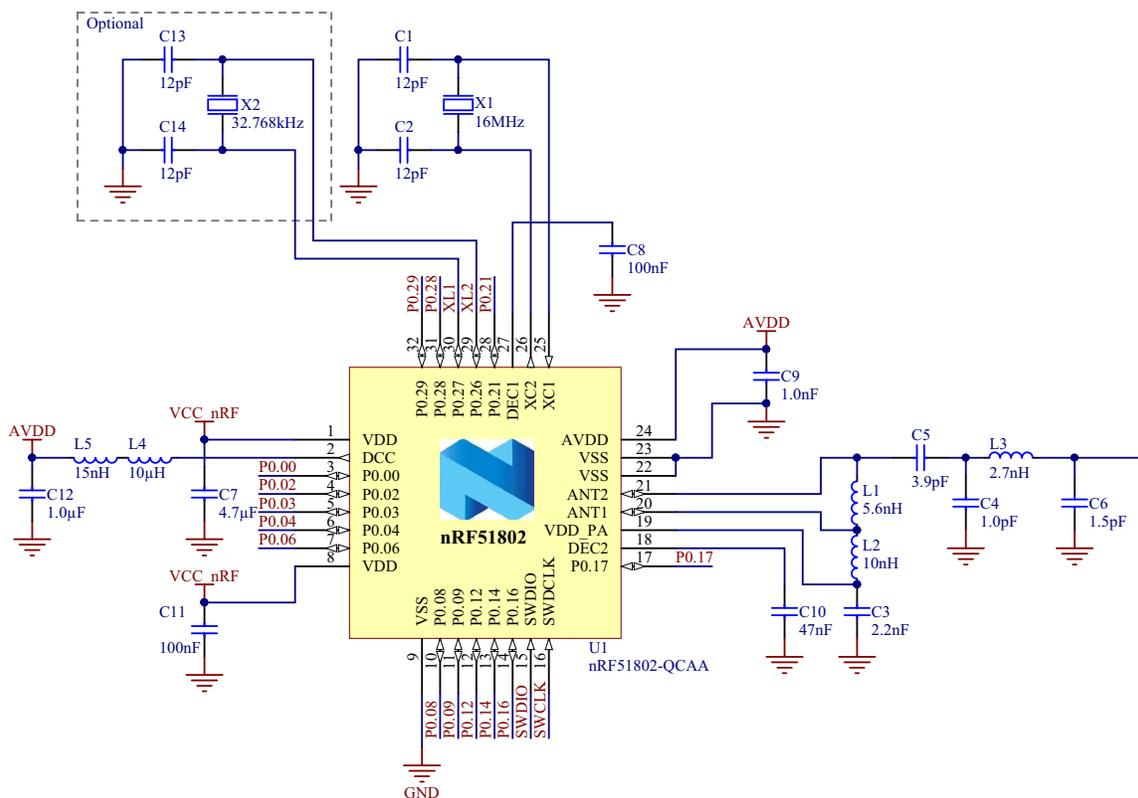
**Figure 24** QCAA QFN32 with DC/DC converter setup
