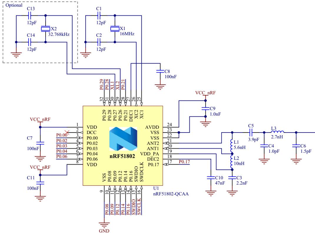
**Figure 22** QCAA QFN32 with internal LDO setup
