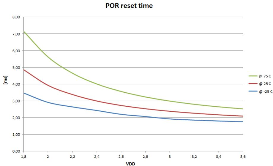
**Figure 9** Power on reset time (Test level 2)
