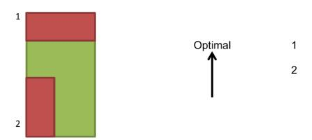
The antenna should be aligned with the pcb edge if possible. It is also important to align pin 1, 2, 3 and 4 along the outer side of the pcb, and ideally close to a corner.
