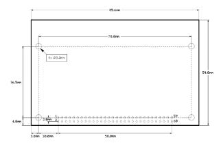
Physical dimensions of the anchor module.
