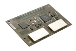
nanoANQ Embedded RTLS Anchor Module
