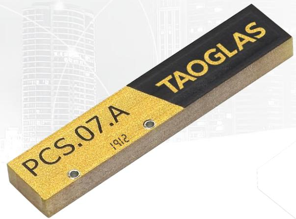
The PCS.07.A is a low profile SMT cellular antenna designed for direct SMT mount on the device PCB. It provides highest efficiency in very small factor 35\*7\*3mm. It is more resistant to detuning compared to other antenna integrations. If tuning is required it can be tuned for the device environment, while there is no need for new tooling. Its rectangular shape and very small size makes it very easy to integrate – can be mounted directly on the edge of the PCB board.
