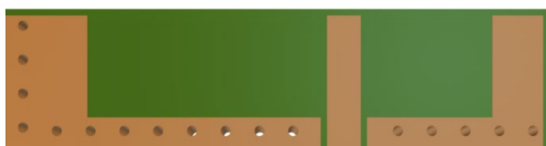
Top View of PCB with Copper Clearance
