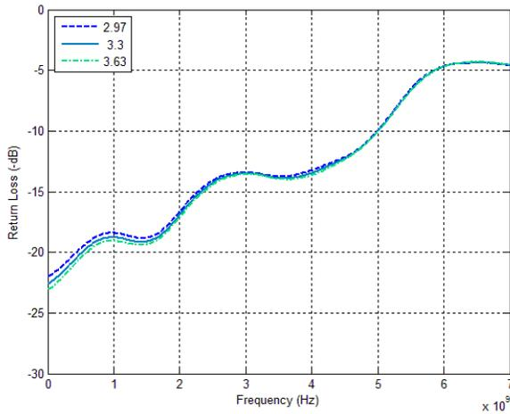
Figure 13. Single-Ended Common Port (A1, A2, X1, X2) Return Loss over Temp
