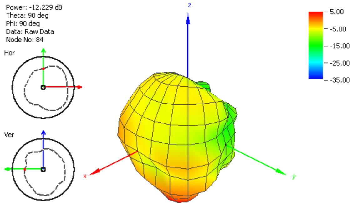
**Figure 8.** Radiation pattern at 900 MHz in Free Space.
