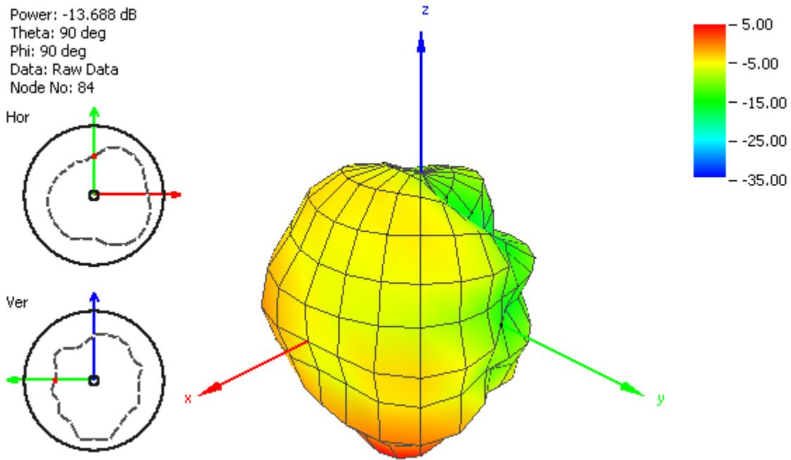
**Figure 9.** Radiation pattern at 915 MHz in Free Space.
