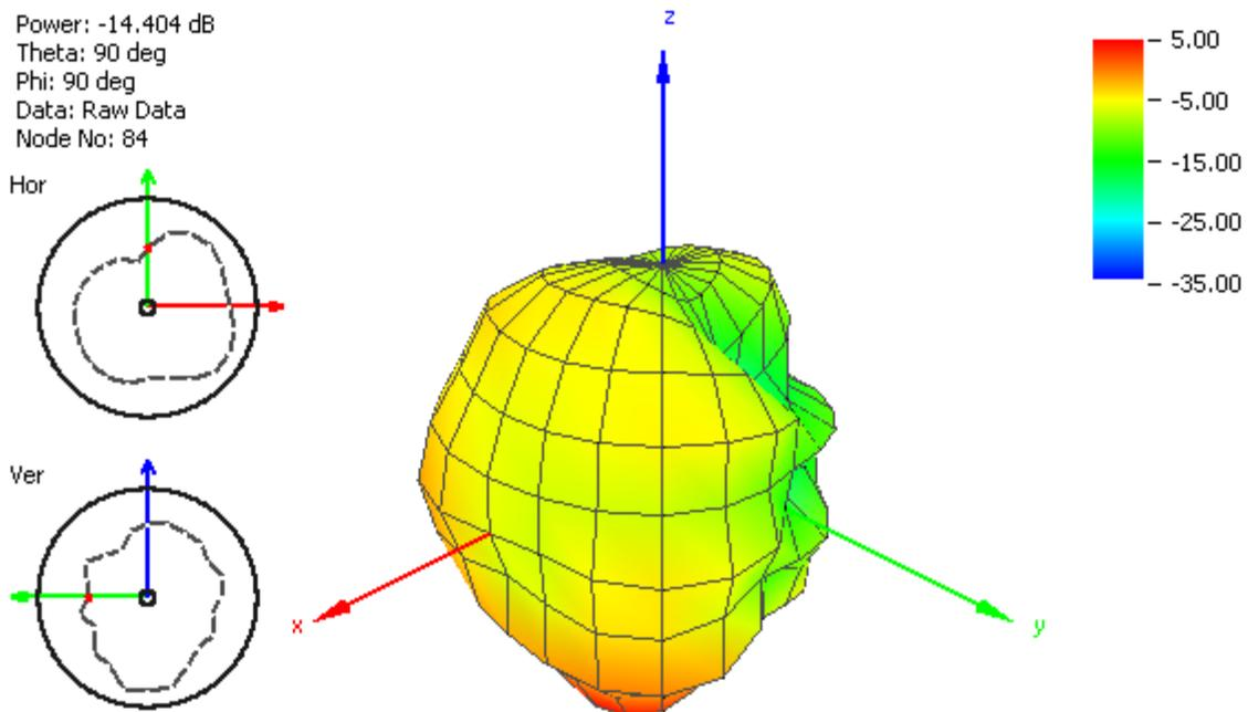
**Figure 10.** Radiation pattern at 930 MHz in Free Space.
