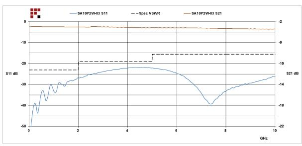
3 dB Fixed Attenuator SMP Male (Plug) to SMP Female (Jack) Up to 10 GHz Rated to 2 Watts, Passivated Stainless Steel Body, 1.4 VSWR from Fairview Microwave is in-stock and available to ship same-day. All of our RF/microwave products are available off-the-shelf from our ISO 9001:2008 certified facilities in Lewisville, Texas. Fairview Microwave is RF on-demand.
