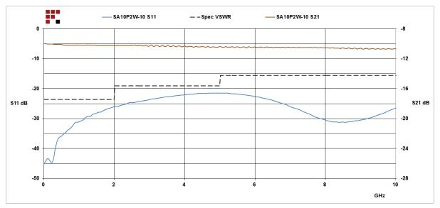
10 dB Fixed Attenuator SMP Male (Plug) to SMP Female (Jack) Up to 10 GHz Rated to 2 Watts, Passivated Stainless Steel Body, 1.4 VSWR from Fairview Microwave is in-stock and available to ship same-day. All of our RF/microwave products are available off-the-shelf from our ISO 9001:2008 certified facilities in Lewisville, Texas. Fairview Microwave is RF on-demand.
