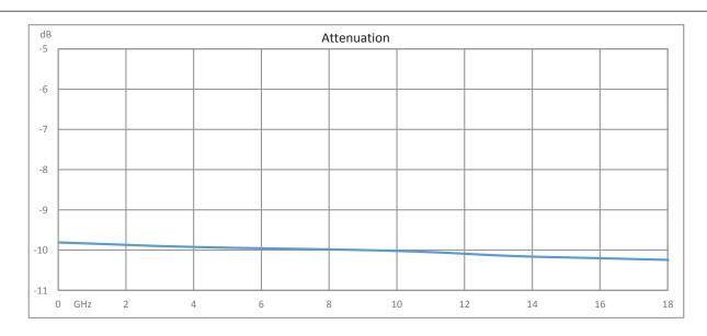
10 dB Fixed Attenuator SMA Male (Plug) to SMA Female (Jack) Up to 18 GHz Rated to 2 Watts, Passivated Stainless Steel Body, 1.35 VSWR from Fairview Microwave is in-stock and available to ship same-day. All of our RF/microwave products are available off-the-shelf from our ISO 9001:2008 certified facilities in Lewisville, Texas. Fairview Microwave is RF on-demand.
